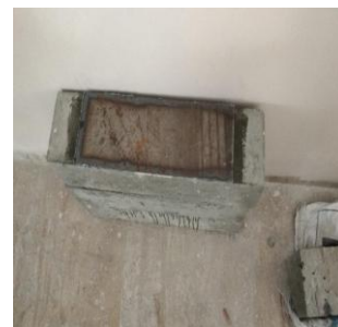
b. Steel plates bonded to the Surface
