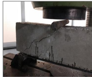
a. Beam with CFRP
