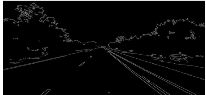
Fig. 5 Canny Edge detection on original Image
