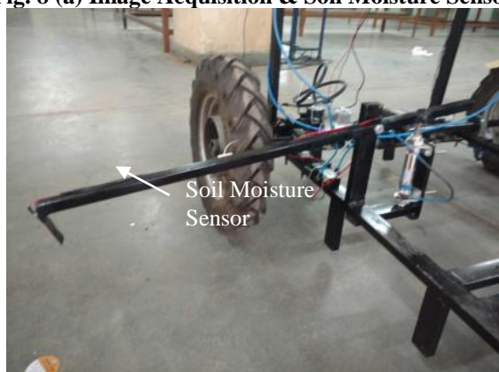
Fig. 8 (b) Soil condition monitoring system
