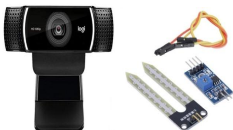
Fig. 8 (a) Image Acquisition & Soil Moisture Sensor
