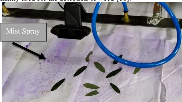
Fig. 12 ( a) Low-density weeds detection & Mist spraying
