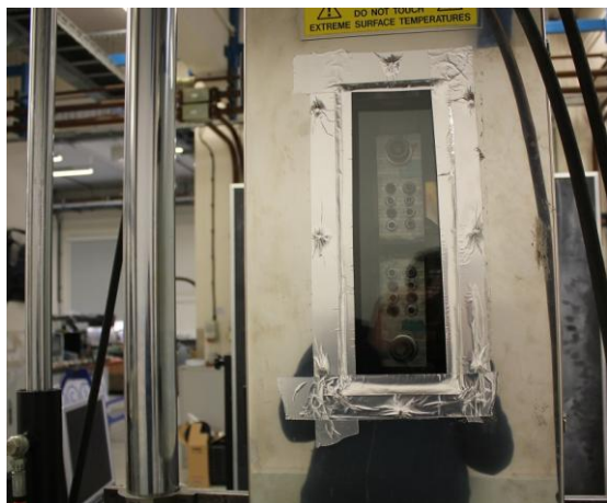
Fig.3. Mechanical testing setup for high temperature (Front view of the chamber)
