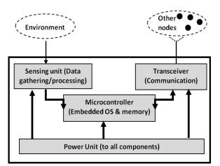
Fig. 1. Hardware Components of a sensor node
