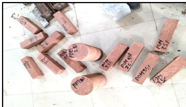
Fig. 6 (b): The trial specimen after 28days curing
