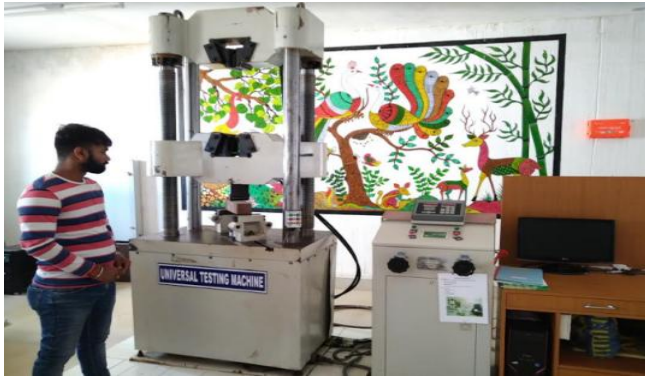
Fig. 5 : Flexural test by UTM (Model BSUT- 100-ZE, Blu star design and manufactured in China)
