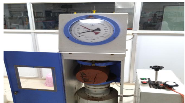
Fig. 4: Split tensile stress of concrete Cylinder with NRM substitute CTM
