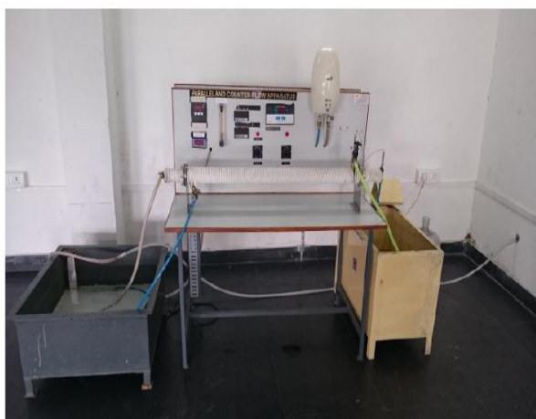
Figure 1 (a) Photographic view of double tube heat exchanging device
