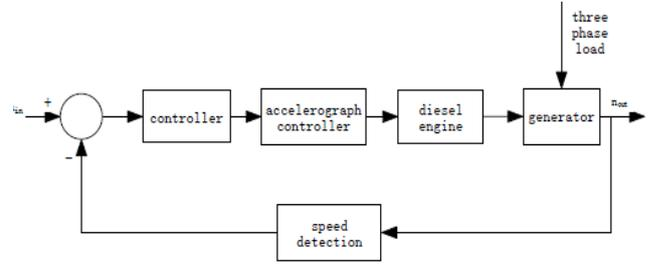
Fig. 2. Block diagram of Diesel engine
