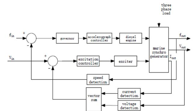
Fig. 4. Block diagram of Speed and Frequency Controller
