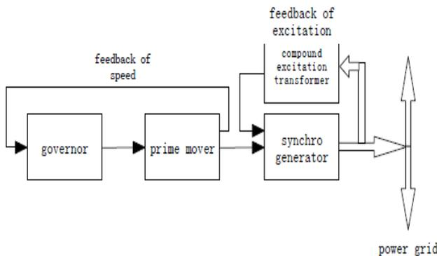
Fig. 1. Block Diagram of diesel generator set
