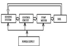
The samples used in the moisture detectors are produced of material that is resistant to corrosion and can be blocked in the soil sample. By evaluating the strength between the probes, the dry and moist voltage levels were calculated and these were paired with output
