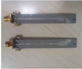
Fig. 6. Implemented RF probes in RF35 substrate.
