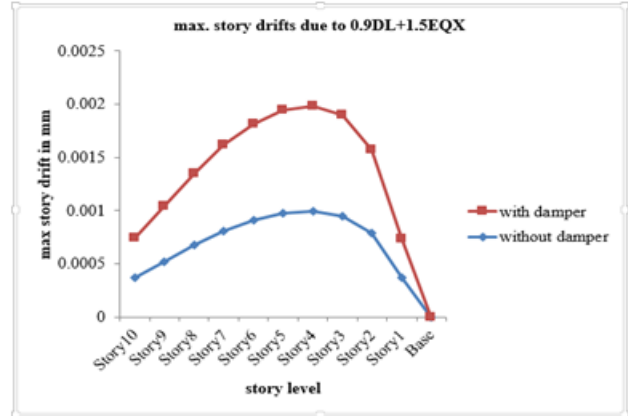
Fig13. Maximum storey drifts due to load combination 0.9DL+1.5EQX in X-direction For SBSC
