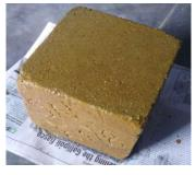
Fig. 9 Acid attack on cube
