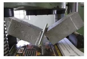
Fig. 8 Flexural test for prism
