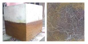
Fig. 10 Sulphate attack on cube
