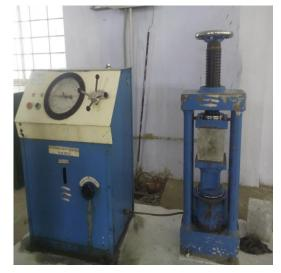
Fig. 7 Compression testing machine
