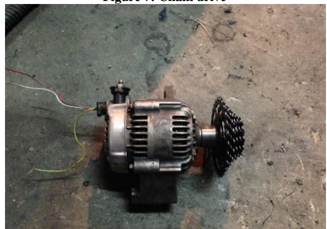
Figure 8: Alternator connected with driven sprocket
