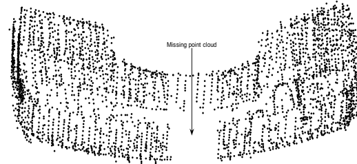
Figure 1 Cloud data obtained after measurement with CMM
