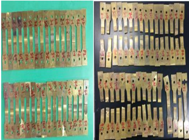
Figure 5: Tensile Test Specimens before and After Test
