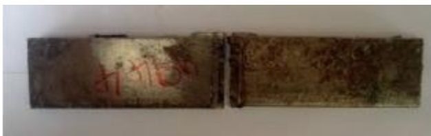
Fig.10 Tensile specimen after fracture.
