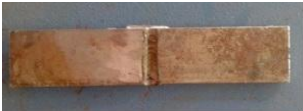
Fig.9 Tensile specimen before fracture
