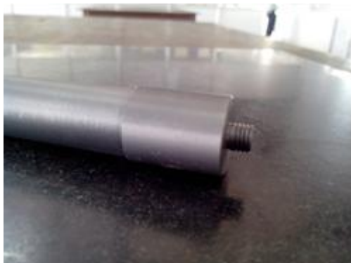
Fig.3 FSW Tool after Machining
