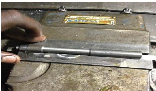
Fig.2. Horizontally placed lever for drilling.
