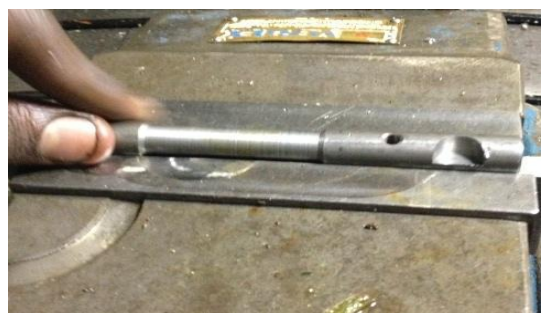
Fig.3. Angularly placed lever for slot milling.
