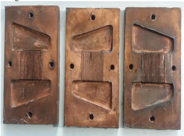
Fig.1 MCHS Original Test pieces copper material.
