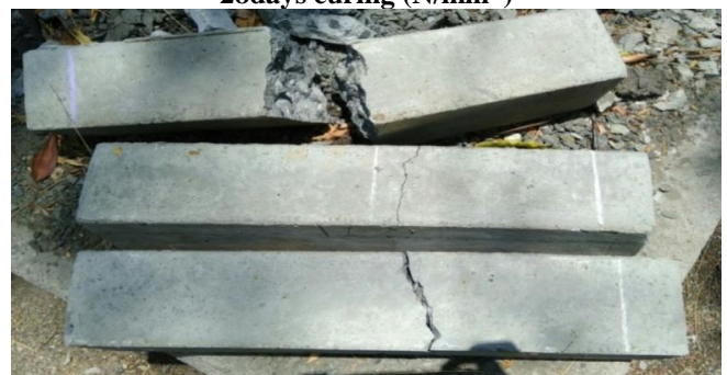
Fig. 8. Tested prism specimen
