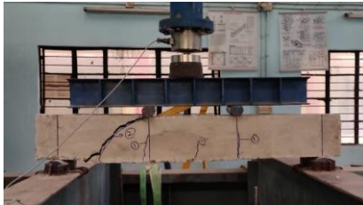
Fig. 13. Failure of RC Beam
