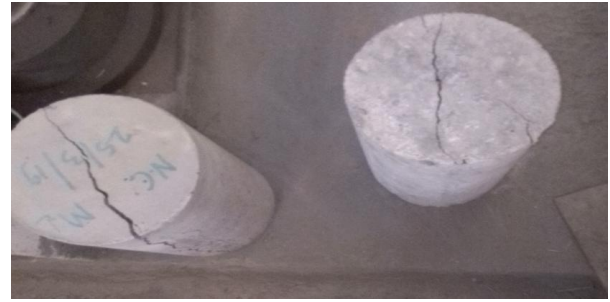
Fig. 6. Tested cylindrical specimen
