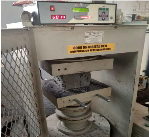
Fig. 4. Testing cubical specimen
