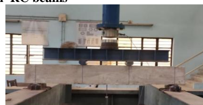
Fig. 12. Test setup of RC Beam
