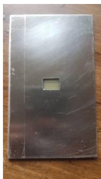
Fig. 3. Bottom view of fabricated antenna with slot in a homogeneous substrate.
