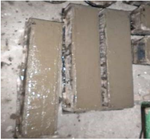
Fig D.1: Casting of Prism Specimens
