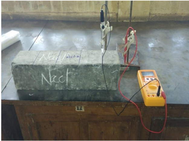
Figure 4. Prediction of Corrosion Levels by OCP Method
