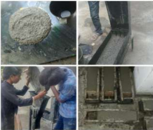
Figure 1. Preparation and Casting of Specimens
