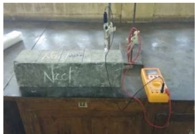
Figure 4 . Prediction of Corrosion Levels by OCP Method
