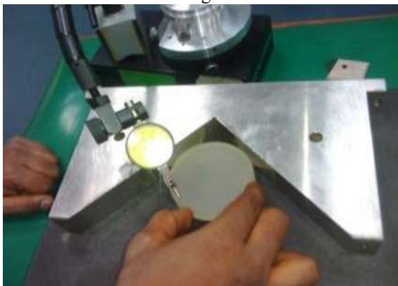
Fig.6 Semi finished lens testing on existing device
