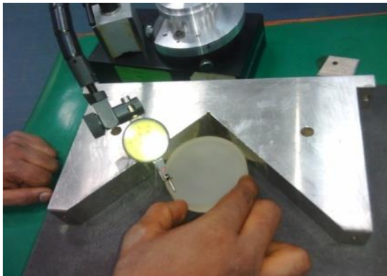
Fig.6 Semi finished lens testing on existing device
