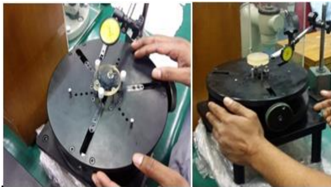
Fig.7 Semi finished lens testing on developed Prototype fixture
