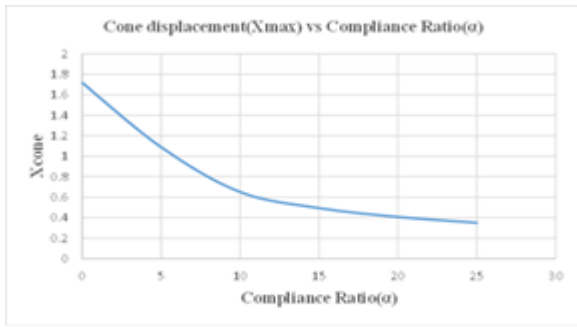
Fig.10. Cone Displacement for Different Compliance Ratios
