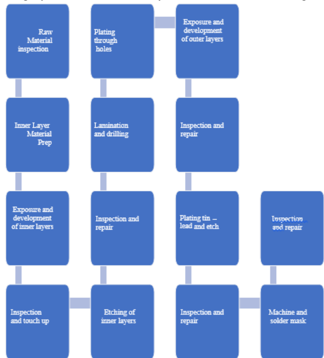
Fig.1: Printed Circuit Board Manufacturing Flow Diagram
