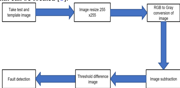
Fig.7: Block Diagram of the Defect Detection in PCB
