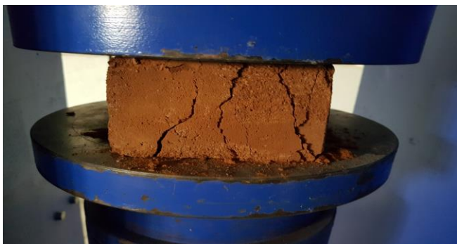
Fig 2. 9: Crushing Strength or Compressive Strength Test on Bricks
