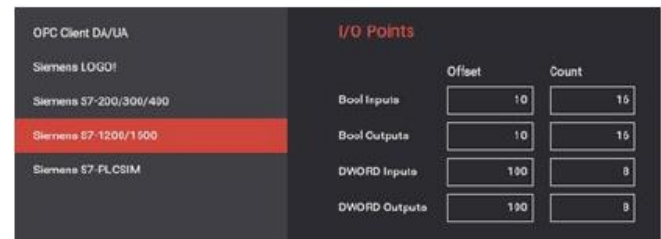
Fig. 3: Configuration in Factory I/O Software of PLC S7-1214 DC/DC/DC
