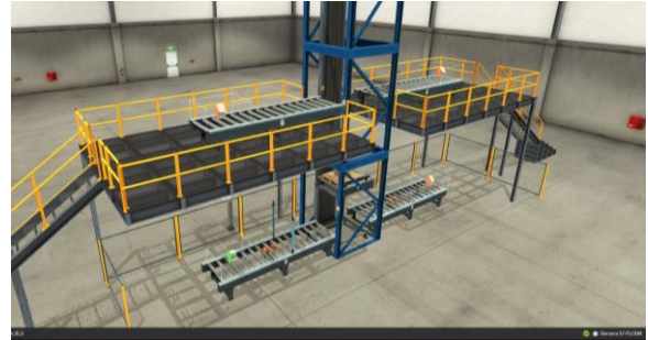
Fig. 2: Designed Sorting Line with lift in Factory I/O Environment
