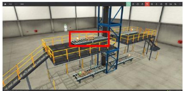
Fig. 13: Representation of the Code Shown in Fig. 14. Made in Factory I/O Software
